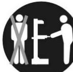
The log splitter must be used by one person alone.
