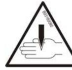
Danger of cutting or crushing of the hand: never touch hazardous areas while the wedge is moving.
