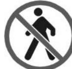
it is forbidden to stand in the range of action of the machine. apart from the operator, no other person or animal may be present within a radius of 5 metres from the machine.
