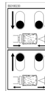
Two hands control: activating both the levers downwards, the wedge will start working and cut the log. Once the log is splitted, push the levers upwards in order to bring the wedge in the upper position, ready to a new work cycle
