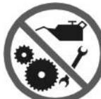
it is forbidden to carry out any maintenance work or to renew parts on the machine when it is running.
