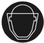
it is obligatory at all times to wear goggles which protects the eyes against chips and splinters which may be produced during work.
